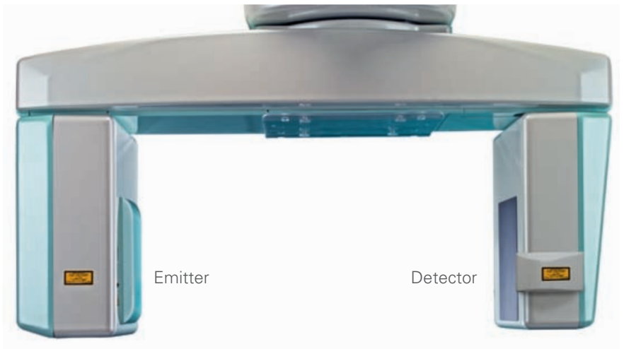
Figure 1: The principle behind the CBCT technique, as its name implies, is a cone-shaped X-ray beam with the X-ray source and detector rotating around a point of interest in the patient. This figure shows a rotating gantry with x-ray source (so-called emitter) and detector attached to it.
